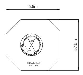
SAFETY SURFACING AREA 24.6m<sup>2</sup> PERIMETER 18m HIC 2.1m
