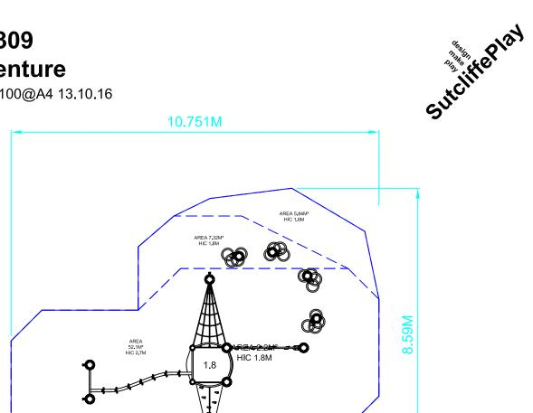
SAFETY SURFACING AREA 61.6M<sup>2</sup> PERIMETER 32.4M HIC 1.8M - 9.5M<sup>2</sup> HIC 2.7M - 52.1M<sup>2</sup>
