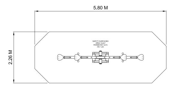
SAFETY SURFACING AREA 12.4m<sup>2</sup> PERIMETER 14.7m HIC 1.3m
