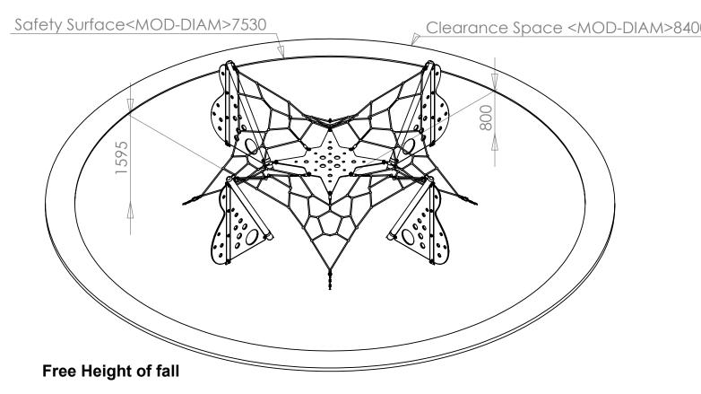
The maximum height at which a child can stand, and fall unimpeded, is 1.595m this is considered to be the free height of fall according to BS-EN 1176 part 11 section 4.3. And therefore a suitable 7.53 metre, circle, Rubber safety surface as shown above, is needed. See table below for recomended Surface Types and Depths:
