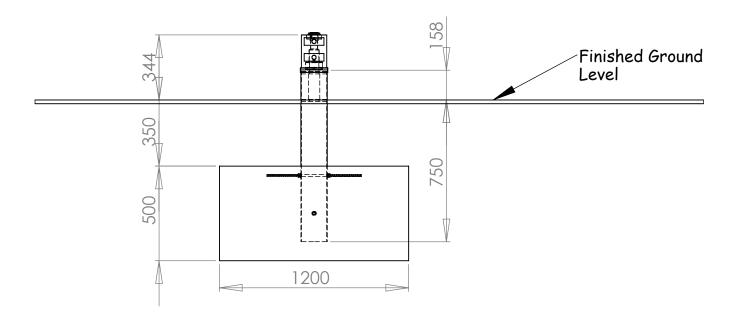
The foundation should be left for approximately seven days to achieve maximum strength prior to assembling the remaining elements.
