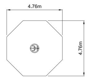
SAFETY SURFACING AREA 19m<sup>2</sup> PERIMETER 12m HIC 0.5m
