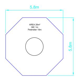
SAFETY SURFACING AREA 28m<sup>2</sup> PERIMETER 19m HIC 1m
