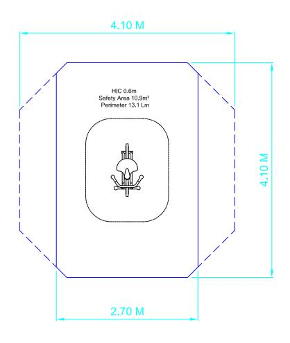
SAFETY SURFACING OUTER AREA 10.9M<sup>2</sup> OUTER PERIMETER 13.1M HIC 0.6M PRODUCT SPECIFICS
