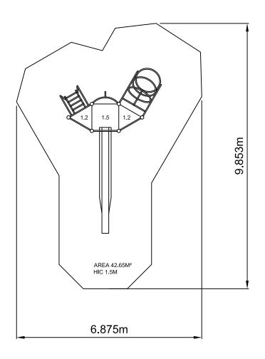
SAFETY SURFACING AREA 42.65m<sup>2</sup> PERIMETER 27.9m HIC 1.5m
