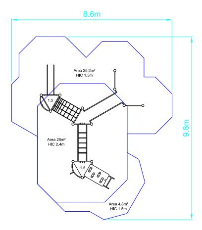
SAFETY SURFACING AREA 58m<sup>2</sup> PERIMETER 33.5m HIC 1.5m 30m<sup>2</sup> HIC 2.4m 28m<sup>2</sup>
