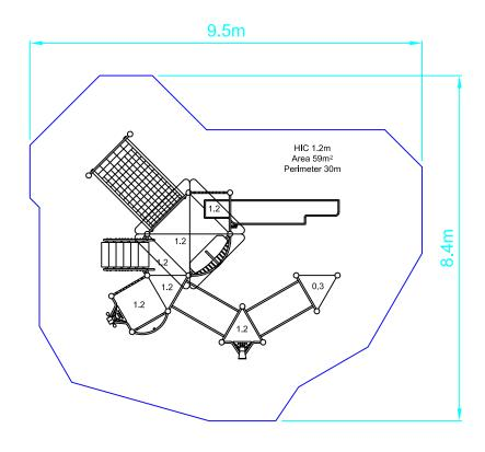
SAFETY SURFACING AREA 59m<sup>2</sup> PERIMETER 30m HIC 1.2m
