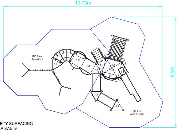
SAFETY SURFACING AREA 87.5m<sup>2</sup> PERIMETER 39m HIC 1.2m 41.5m<sup>2</sup> HIC 2.4m 46m<sup>2</sup>
