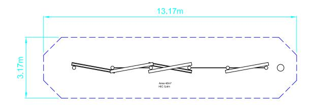
SAFETY SURFACING AREA 40m<sup>2</sup> PERIMETER 30.5m HIC 0.4m
