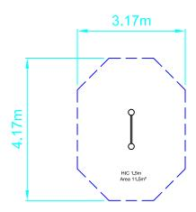
SAFETY SURFACING AREA 11.5m<sup>2</sup> PERIMETER 12.5m HIC 1.5m
