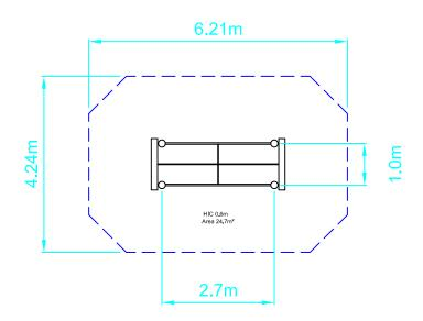
SAFETY SURFACING NONE REQUIRED MINIMUM UE ZONE SHOWN AREA 24.7m<sup>2</sup> PERIMETER 18m HIC 0.6m PRODUCT SPECIFICS
