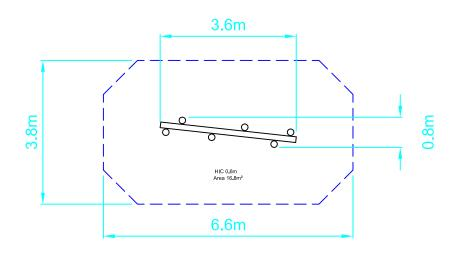
SAFETY SURFACING NON REQUIRED MINIMUM USE ZONE SHOWN AREA 23.5m<sup>2</sup> PERIMETER 18.7m HIC 0.6m PRODUCT SPECIFICS
