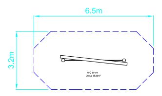
SAFETY SURFACING AREA 18.8m<sup>2</sup> PERIMETER 17m HIC 0.4m
