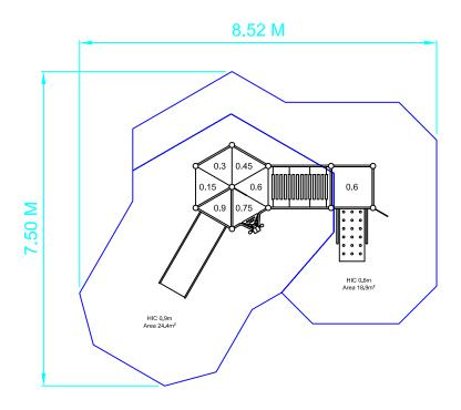
SAFETY SURFACING Area 43.3m<sup>2</sup> Perimeter 27.3m HIC 0.6m - AREA 18.9m<sup>2</sup> HIC 0.9m - AREA 24.4m<sup>2</sup> SAFETY SURFACING OPTIONAL
