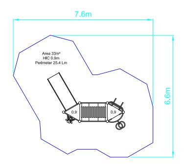
SAFETY SURFACING AREA 33m<sup>2</sup> PERIMETER 25.4m HIC 0.9m
