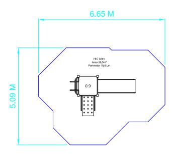
SAFETY SURFACING AREA 26.5m<sup>2</sup> PERIMETER 19.8m HIC 0.9m
