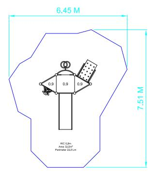
SAFETY SURFACING AREA 32.5M<sup>2</sup> PERIMETER 22.5M HIC 0.9M - 32.5M<sup>2</sup>
