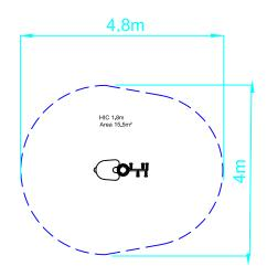
SAFETY SURFACING AREA 15.5m<sup>2</sup> PERIMETER 14.1m
